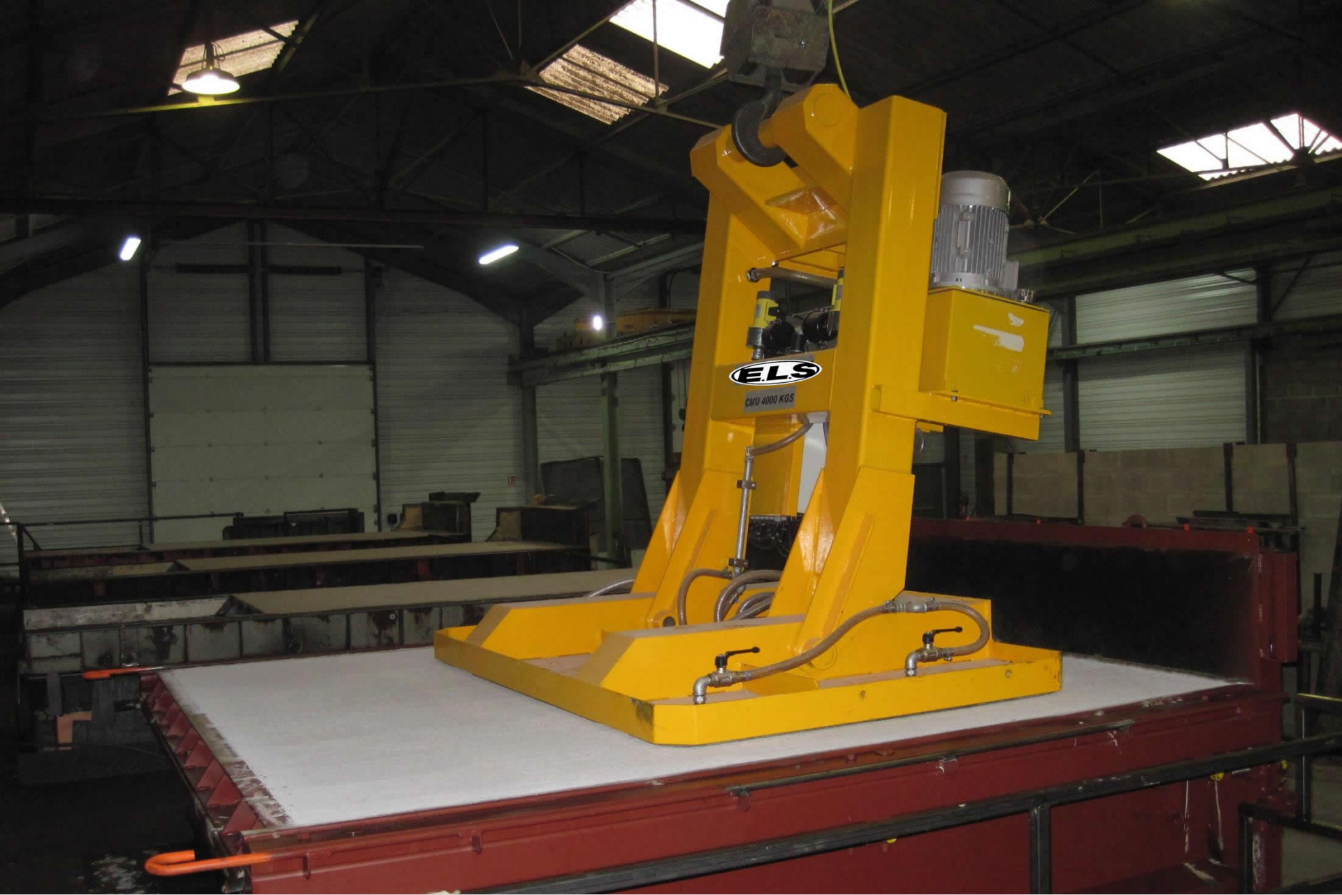
Concrete cast demoulding 3m Long & 2,5m wide & 5 T
