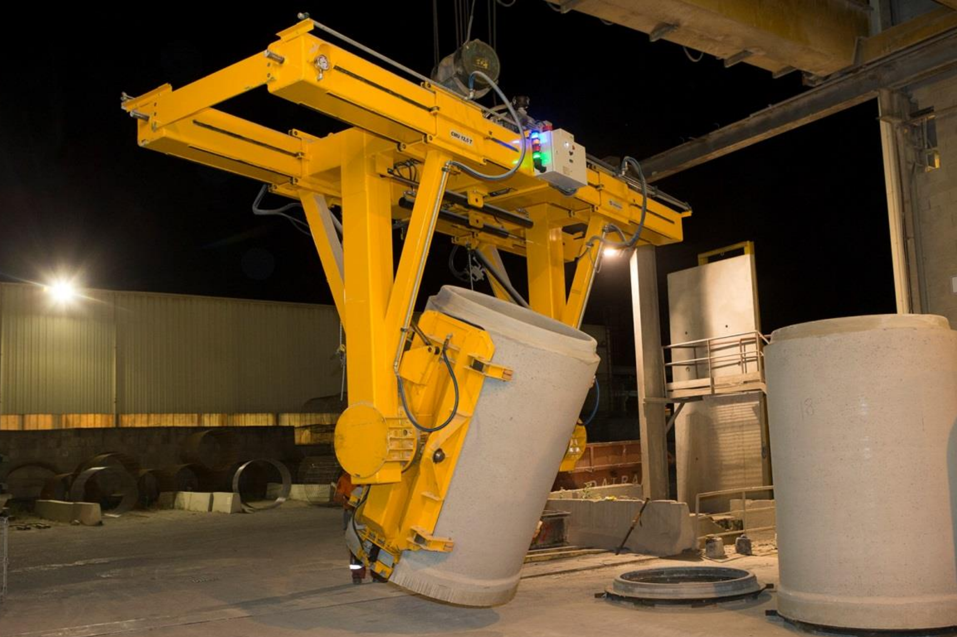
Tank cast, \text{Ø}1,7\text{m} & Height 2,7\text{m} & 8 T
